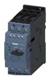
CIRCUIT BREAKER, SIZE S2, FOR MOTOR PROTECTION, CLASS 20, A-RELEASE 42...52A, N-RELEASE 741A, SCREW TERMINAL, STANDARD BREAKING CAPACITY W. TRANSV. AUX. SWITCH 1NO+1NC
