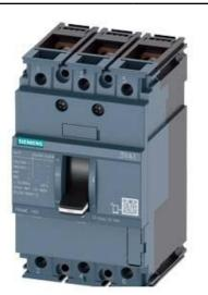
CIRCUIT BREAKER 3VA1 IEC FRAME 160 BREAKING CAPACITY CLASS S ICU=36KA @ 415 V 3-POLE, LINE PROTECTION TM210, FTFM, IN=160A OVERLOAD PROTECTION IR=160A FIXED SHORT CIRCUIT PROTECTION II=10 X IN BUSBAR CONNECTION
