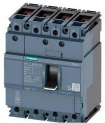
CIRCUIT BREAKER 3VA1 IEC FRAME 160 BREAKING CAPACITY CLASS N ICU=25KA @ 415 V 4-POLE, LINE PROTECTION TM210, FTFM, IN=80A OVERLOAD PROTECTION IR=80A FIXED SHORT CIRCUIT PROTECTION II=10 X IN NEUTRAL PROTECTION 100% BUSBAR CONNECTION
