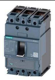
CIRCUIT BREAKER 3VA1 IEC FRAME 160 BREAKING CAPACITY CLASS H ICU=70KA @ 415 V 3-POLE, LINE PROTECTION TM220, ATFM, IN=80A OVERLOAD PROTECTION IR=56A ...80A SHORT CIRCUIT PROTECTION II=10 X IN BUSBAR CONNECTION
