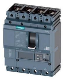
CIRCUIT BREAKER 3VA2 IEC FRAME 160 BREAKING CAPACITY CLASS C ICU=110KA @ 415 V 4POLE, LINE PROTECTION ETU850, LSI, IN=160A OVERLOAD PROTECTION IR=64A ...160A SHORT CIRCUIT PROTECTION ISD=0,6..10X IN, II=1,5..10X IN NEUTRAL PROTECTION ADJUSTABLE (OFF, UPTO 100%) BUSBAR CONNECTION
