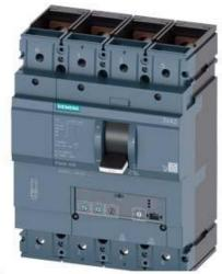
CIRCUIT BREAKER 3VA2 IEC FRAME 630 BREAKING CAPACITY CLASS M ICU=55KA @ 415 V 4-POLE, LINE PROTECTION ETU320, LI, IN=400A OVERLOAD PROTECTION IR=160A ...400A SHORT CIRCUIT PROTECTION II=12 X IN NEUTRAL PROTECTION ADJUSTABLE(OFF,50%,100%) BUSBAR CONNECTION
