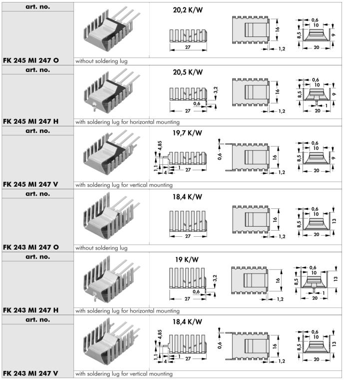
material:copper (Cu)material thickness:0.6 mmsurface treatment:solderable
