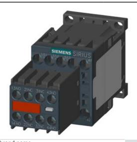
CONTACTOR, AC-3, 4KW/400V, 2NO+2NC, AC 230V, 50/60 HZ, 3-POLE, SZ S00 SCREW TERMINAL PERMANENT AUX. SWITCH FOR SUVA APPLICATIONS
