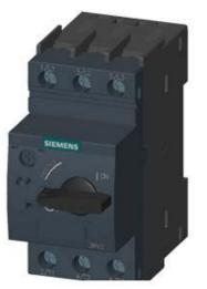
SPECIAL TYPE CIRCUIT BREAKER SIZE S0, FOR TRANSFORMER PROTECTION A-RELEASE 13...20A, SHORT-CIRCUIT RELEASE 325A, SCREW TERMINAL, STANDARD SWITCHING CAPACITY AMBIENT TEMPERATURE -50 DEGREES C 500 SWITCHING CYCLES
