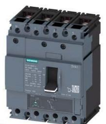
CIRCUIT BREAKER 3VA1 IEC FRAME 160 BREAKING CAPACITY CLASS M ICU=55KA @ 415 V 4-POLE, LINE PROTECTION TM220, ATFM, IN=125A OVERLOAD PROTECTION IR=87,5A ...125A SHORT CIRCUIT PROTECTION II=10 X IN NEUTRAL PROTECTION 50% BUSBAR CONNECTION
