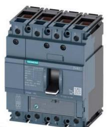
CIRCUIT BREAKER 3VA1 IEC FRAME 160 BREAKING CAPACITY CLASS M ICU=55KA @ 415 V 4-POLE, LINE PROTECTION TM220, ATFM, IN=160A OVERLOAD PROTECTION IR=112A ...160A SHORT CIRCUIT PROTECTION II=10 X IN NEUTRAL PROTECTION 50% CABLE CONNECTION
