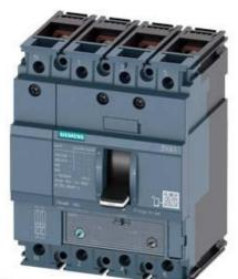
CIRCUIT BREAKER 3VA1 IEC FRAME 160 BREAKING CAPACITY CLASS N ICU=25KA @ 415 V 4-POLE, LINE PROTECTION TM240, ATAM, IN=80A OVERLOAD PROTECTION IR=56A ...80A SHORT CIRCUIT PROTECTION II=5 X IN NEUTRAL PROTECTION 100% BUSBAR CONNECTION
