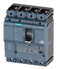
CIRCUIT BREAKER 3VA2 IEC FRAME 160 BREAKING CAPACITY CLASS M ICU=55KA @ 415 V 4POLE, LINE PROTECTION ETU350, LSI, IN=63A OVERLOAD PROTECTION IR=25A ...63A SHORT CIRCUIT PROTECTION ISD=1,5... 10 X IR, II=12 X IN NEUTRAL PROTECTION ADJUSTABLE(OFF,100%) BUSBAR CONNECTION
