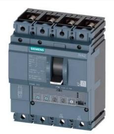
CIRCUIT BREAKER 3VA2 IEC FRAME 250 BREAKING CAPACITY CLASS C ICU=110KA @ 415 V 4POLE, LINE PROTECTION ETU330, LIG, IN=250A OVERLOAD PROTECTION IR=100A ...250A SHORT CIRCUIT PROTECTION II=1,5...10 X IN NEUTRAL PROTECTION ADJUSTABLE(OFF,50%,100%) GROUNDFAULTPROTECTION IG=0,2... 1 X IN, TG=0,1/0,3MS BUSBAR CONNECTION
