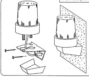
The FX4 is suitable for use with LT Series Beacons. The bracket is made of black ABS and enables these beacons to be mounted on a wall or panel.
