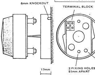
The FX2 is suitable for use with L, LP & LT Series beacons. The base is made of black ABS. It may be fitted to either a conduit box or wall. Accessories are included to enable the beacon to be bayonet fitted onto the base.
