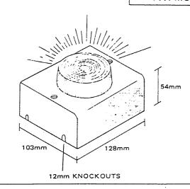
The FX1 is suitable for use with L, LP & LT Series beacons. It is made of grey, high impact polystyrene. Mounting accessories and terminal block are included. The box is suitable for internal wall or ceiling surface mounting of beacons.
