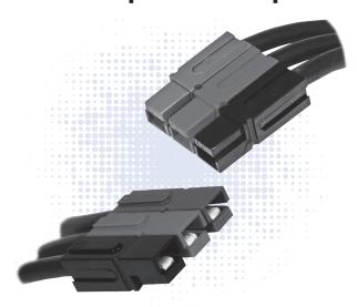
PP120 series Powerpole® housings are designed to accommodate up to 1/0 (50 mm²) wires and handle high currents up to 240 amps. Reducing bushings allow PP120 to accept down to #8 (10 mm²) wires. Multiple colors of stackable housings combine with low resistance flat wiping technology to offer powerful connection capability.
