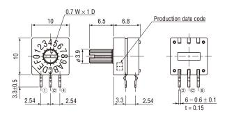
Unless otherwise specified, tolerance:  $\pm$  0.3 (Unit: mm)
