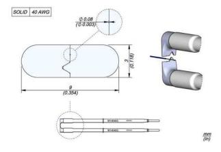
W14040G is specially designed for stripping high-temperature wire insulationsmade of thermostable materials such as Teflon\*, Kapton\*, silicone rubber, etc, of 40 AWG (0.08 mm / 0.0031 in).
