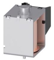
Accessory 3WA/3WL Closing coil (CC) / Shunt trip (ST), 100% OP 24-30 V DC for continuous duty
