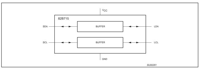
Figure 1. Block Diagram: 82B715
