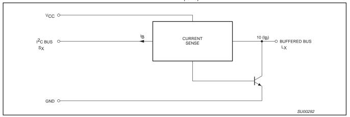
Figure 2. Equivalent Circuit: One Half 82B715
