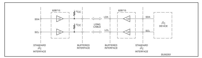
Figure 3. Minimum Sub-System with 82B715
