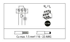
The remote status indicator (SPDT contact) shall be connected to NEC class 2 circuits only!
