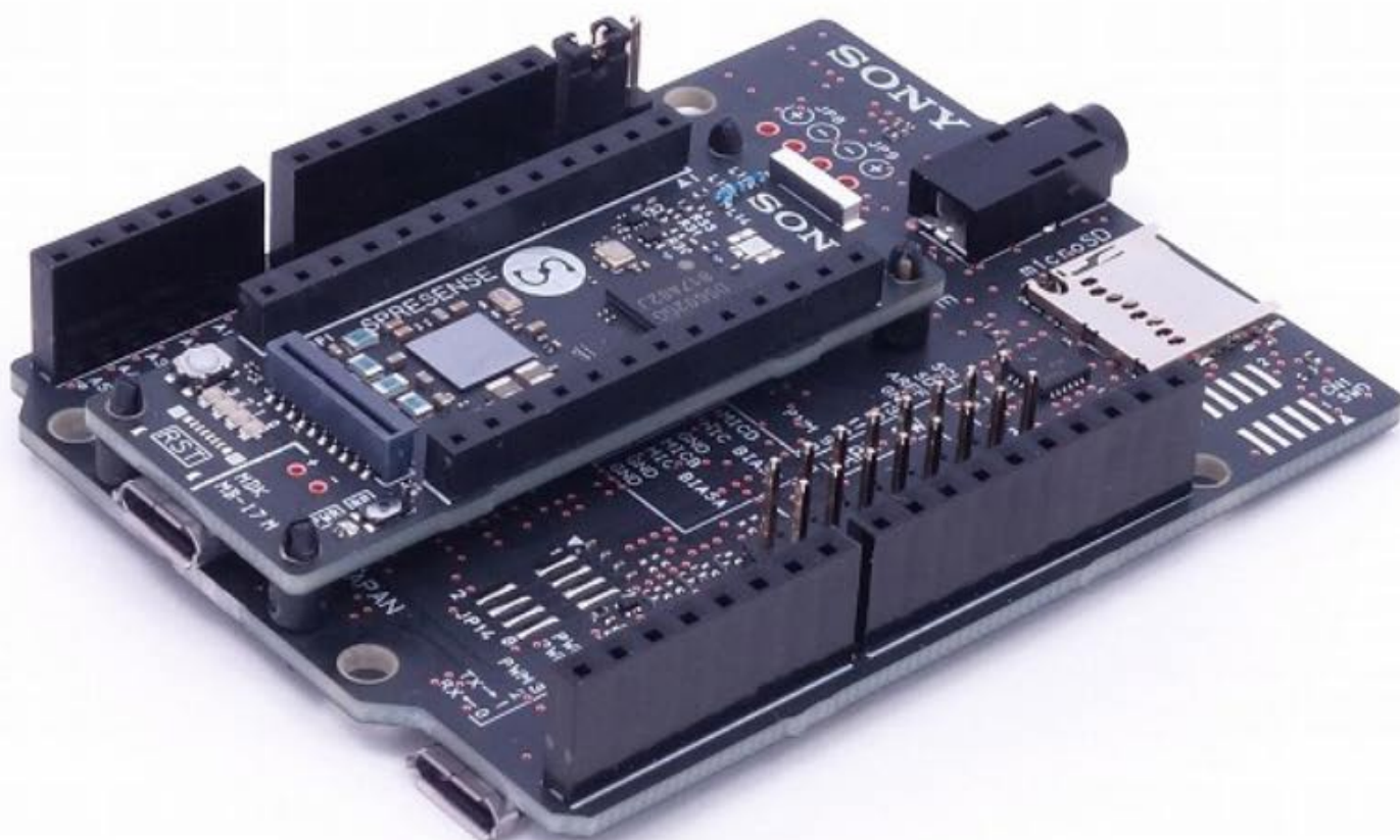
Figure 1. Extension board at the bottom and the main board mounted on top.
