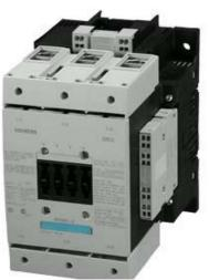
CONTACTOR, 55KW/400V/AC-3 AC(40...60HZ)/DC OPERATION UC 500-550V AUXILIARY CONTACTS 2NO+2NC 3-POLE, SIZE S6 WITH BOX TERMINALS CONVENTIONAL OPERATING MECHAN. CAGE CLAMP CONNECTION
