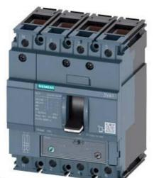
CIRCUIT BREAKER 3VA1 IEC FRAME 160 BREAKING CAPACITY CLASS H ICU=70KA @ 415 V 4-POLE, LINE PROTECTION TM240, ATAM, IN=100A OVERLOAD PROTECTION IR=70A ...100A SHORT CIRCUIT PROTECTION II=5...10 X IN NEUTRAL UNPROTECTED CABLE CONNECTION
