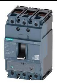
CIRCUIT BREAKER 3VA1 IEC FRAME 160 BREAKING CAPACITY CLASS N ICU=25KA @ 415 V 3-POLE, LINE PROTECTION TM240, ATAM, IN=40A OVERLOAD PROTECTION IR=28A ...40A SHORT CIRCUIT PROTECTION II=5...10 X IN CABLE CONNECTION
