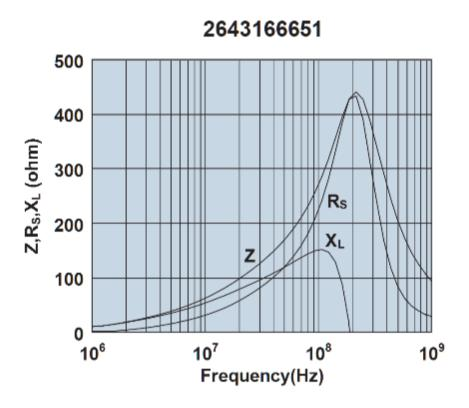
Impedance, reactance, and resistance vs. frequency.
