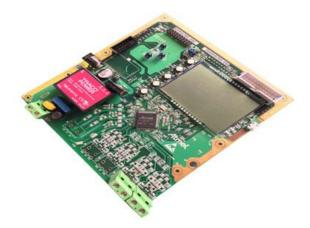
The ATSAM4CMS32-DB demonstration board uses Atmel ATSAM4CMS32 to demonstrate the high accuracy single-phase energy metering functions. The ATSAM4CMS32 is an integrated single-phase Energy Metering SoC with 100MHz, dual-core Cortex-M4 ARM processor cores. The board is ETSI format compliant and is designed to interface with CT, Rogowski and Shunt current sensors. The board can interface with ZigBee and PLC communication modules from Atmel.
