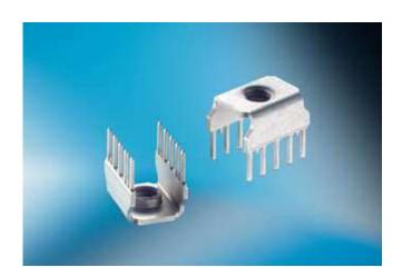
The ERNI Power Tap is designed to bring power to printed circuit board applications. It allows for wire-to-board connections with common terminals. The 10 pin version has five solder pins per row with a two-row PCB layout. The operating current is determined by characteristics of the PCB and the cable termination. This power supply cable can be connected with a screw mount terminal accomodating M3, M4, 6-32UNC or 8-32UNC screws.
