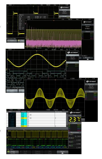
After capturing a serial bus communication, you can easily perform a search-and-navigation operation based on specific criteria of your interest. Note, the digital channels and serial protocol analysis cannot be used simultaneously.
