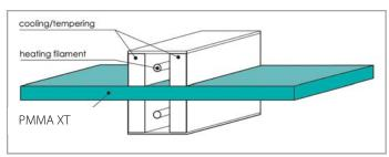
Extended heating is carried out by filaments or heating rods. The heating time depends on the equipment employed and will rise considerably according to increased material thickness.
