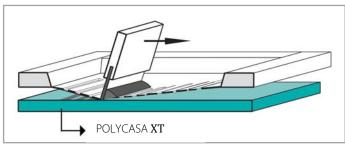
Distortion screen printing allows the flat sheet to be formed after printing into a three dimensional article with correct print register. Allowance must be made for "stretching" of the image when designing the graphics.
