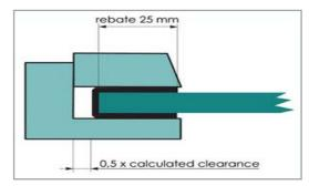
The linear change must be allowed during the sheet's storage time. The maximum expected value of linear deformation depends on the temperature used when mounting the sheets.
