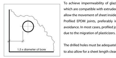
To achieve impermeability of glazing to rain water, only sealing agents shall be used which are compatible with extruded acrylic sheet Construction and sealing material must allow the movement of sheet inside the profiles due to dimensional changes of sheet. Profiled EPDM joints, preferably in white, have proven to be successful in heat loss avoidance. In most cases, profiled joints of non-rigid PVC and PUR foam are incompatible,
