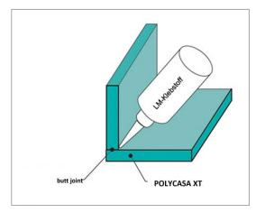
Polymerisation adhesives are also suitable for large and uneven bonding surfaces. Planar bonding is possible.
