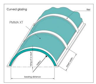
to plane roofing, as an increased self-rigidity of the sheet is achieved due to the change in geometry.
