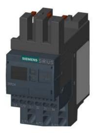
CURRENT MONITORING RELAY MOUNTABLE ON CONT. 3RT2, SZ. S0, APPARENT/ACTIVE CURR. MONIT. 4 - 40A, 20-400 HZ, 3-PH., SUPPLY 24 V DC, 1 CO CONTACT, MONITORING F. CURRENT OVER-/UNDERSHOOT, CURRENT ASYMMETRY, PHASE FAILURE / WIRE BREAK, PHASE SEQUENCE, FAULT CURRENT, BLOCKING CURRENT, SWITCHING CYCLE/OP. HOURS COUNTER, WARNING/ALARM THRESHOLDS, AUTO OR MANUAL RESET ON-DELAY 0-999.9 S OFF-DELAY 0-999.9 S RECLOSING DELAY 0-999.9MIN SPRING-LOADED CONNECTION
