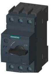
CIRCUIT-BREAKER SZ S0, FOR MOTOR PROTECTION, CLASS 10, A-REL. 0.55...0.8A, N-REL. 10A SCREW CONNECTION, STANDARD SW. CAPACITY
