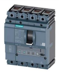
CIRCUIT BREAKER 3VA2 IEC FRAME 100 BREAKING CAPACITY CLASS H ICU=85KA @ 415 V 4POLE, LINE PROTECTION ETU350, LSI, IN=63A OVERLOAD PROTECTION IR=25A ...63A SHORT CIRCUIT PROTECTION ISD=1,5... 10 X IR, II=12 X IN NEUTRAL PROTECTION ADJUSTABLE(OFF,100%) CABLE CONNECTION
