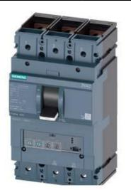
CIRCUIT BREAKER 3VA2 IEC FRAME 400 BREAKING CAPACITY CLASS C ICU=110KA @ 415 V 3-POLE, LINE PROTECTION ETU330, LIG, IN=400A OVERLOAD PROTECTION IR=160A ...400A SHORT CIRCUIT PROTECTION II=1,5...10 X IN GROUND-FAULT-PROTECTION IG=0,2... 1 X IN, TG=0,1/0,3MS BUSBAR CONNECTION
