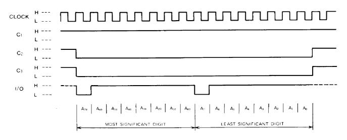
Note 2. The addresses from  $A_{ao}$  to  $A_{77}$  are designated by two one-of-eight coded digits. The above figure shows designation of address  $A_{77}$
