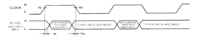
Note 3  $|C_4| \sim |C_3|$  and accept data are interchnageable while the clock is set high.
