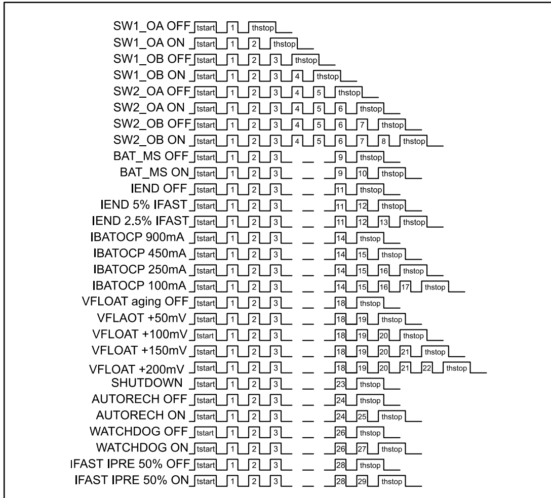
Figure 21: Single wire programming (SW_SEL INPUT)
