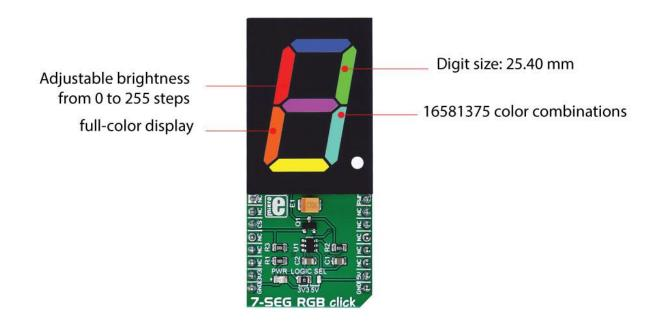
Each segment has R, G, B LEDs that can be adjusted in 255 steps and therefore 16,581,375 color combinations are available for each segment of the digit on the display.
