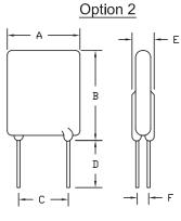
Lead Size: 20 AWG Ø0.81mm Diameter
