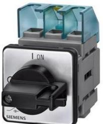
MAIN CONTROL SWITCH 3-POLE IU=32, P/AC-23A AT 400V=11,5KW FRONT MOUNTING FOUR-HOLE MOUNTING KNOB BLACK
