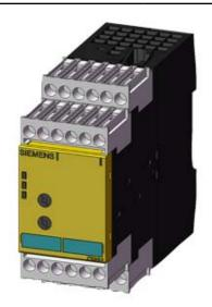
SIRIUS SAFETY RELAY FOR SAFETY-ORIENTED STANDSTILL MONITORING, 24V DC, 45.0MM, SCREW TERMINAL, FK INSTANT.: 3NO 1NC, FK DELAYED: 0, MK: 3, AUTO START, BASIC UNIT, MAX. ACHIEV. CAT. EN954-1: 4, MAX. ACHIEV. SIL TO IEC61508:3,
