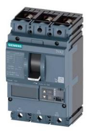
CIRCUIT BREAKER 3VA2 IEC FRAME 100 BREAKING CAPACITY CLASS H ICU=85KA @ 415 V 3POLE, LINE PROTECTION ETU550, LSI, IN=63A OVERLOAD PROTECTION IR=25A ...63A SHORT CIRCUIT PROTECTION ISD=0,6..10X IN, II=1,5..12X IN NEUTRAL PROTECTION OPTIONAL WITH EXT. CT,UPTO 160% BUSBAR CONNECTION
