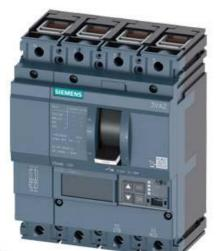
CIRCUIT BREAKER 3VA2 IEC FRAME 100 BREAKING CAPACITY CLASS L ICU=150KA @ 415 V 4POLE, LINE PROTECTION ETU860, LSIG, IN=63A OVERLOAD PROTECTION IR=25A ...63A SHORT CIRCUIT PROTECTION ISD=0,6..10X IN, II=1,5..12X IN NEUTRAL PROTECTION ADJUSTABLE (OFF, UPTO 160%) GROUNDFAULT, SWITCHABLE IG=0,2... 1 X IN, TG=0,050,8MS CABLE CONNECTION
