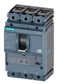
CIRCUIT BREAKER 3VA2 IEC FRAME 160 BREAKING CAPACITY CLASS H ICU=85KA @ 415 V 3POLE, LINE PROTECTION ETU330, LIG, IN=63A OVERLOAD PROTECTION IR=25A ...63A SHORT CIRCUIT PROTECTION II=1,5...12 X IN GROUNDFAULTPROTECTION IG=0,2... 1 X IN, TG=0,1/0,3MS CABLE CONNECTION
