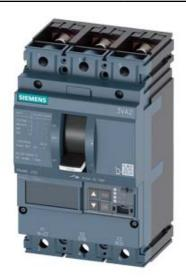
CIRCUIT BREAKER 3VA2 IEC FRAME 250 BREAKING CAPACITY CLASS M ICU=55KA @ 415 V 3POLE, LINE PROTECTION ETU860, LSIG, IN=250A OVERLOAD PROTECTION IR=100A ...250A SHORT CIRCUIT PROTECTION ISD=0,6..10X IN, II=1,5..10X IN NEUTRAL PROTECTION OPTIONAL WITH EXT. CT,UPTO 160% GROUNDFAULT, SWITCHABLE IG=0,2... 1 X IN, TG=0,050,8MS BUSBAR CONNECTION
