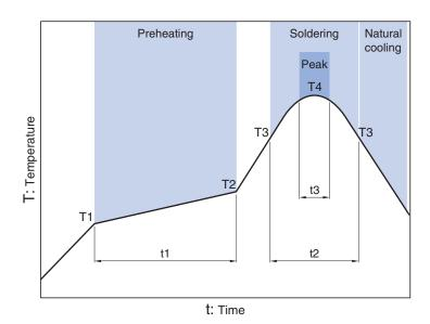
Soldering Preheating Peak Temp. Temp. Temp. Time Time Time T1 T2 **T4** Т3 t3 150°C 180°C 60 to 120s 230°C 30 to 60s 250 to 260°C 10s max.
