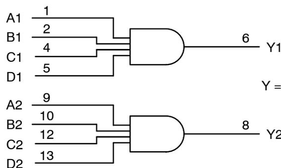
$$Y = A \cdot B \cdot C \cdot D \text{ or } Y = \overline{\overline{A} + \overline{B} + \overline{C} + \overline{D}}$$
