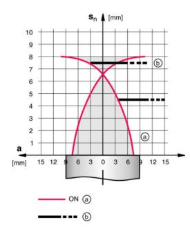
a Inductive switchb Standard measuring plate
