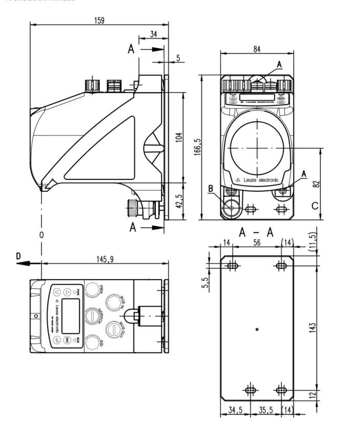
A M 5 screw for alignment
