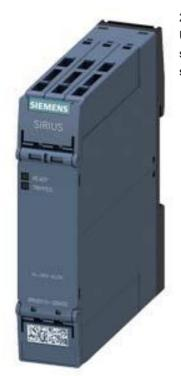
Thermistor motor prot. relay Standard evaluation unit 22.5 mm enclosure Spring-type terminals 2 CO contacts US = 24-240 V AC/DC Auto RESET Suitable for bimetal switches 2 LEDs (READY/TRIPPED) Galvanic separation
