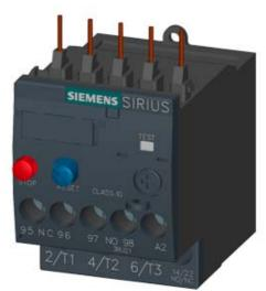
OVERLOAD RELAY 1.8...2.5 A FOR MOTOR PROTECTION SZ S00, CLASS 10, F. MOUNTING ONTO CONTACTOR MAIN CIRCUIT: SCREW TERMINAL AUX. CIRCUIT: SCREW TERMINAL MANUAL-AUTOMATIC-RESET
